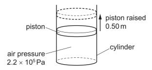
The expansion of the air causes the piston to rise through a vertical distance of 0.50 m, doing 11 kJ of work. Frictional forces are negligible.
