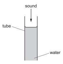
Water is then removed from the tube until a second louder sound is heard.
